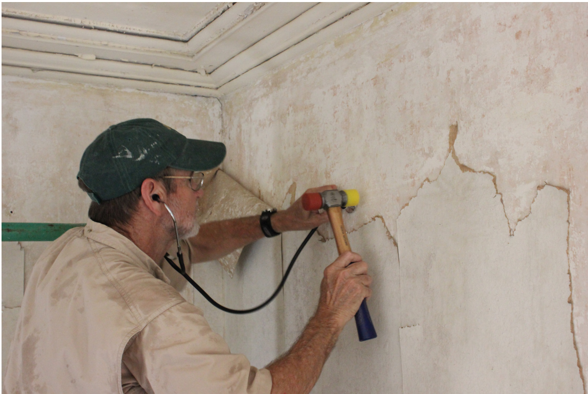
Figure 12: Southeast chamber: A stethoscope and a plastic mallet was used to delicately sound the walls and listen for audible changes, indicating changes in the density of the plaster.
