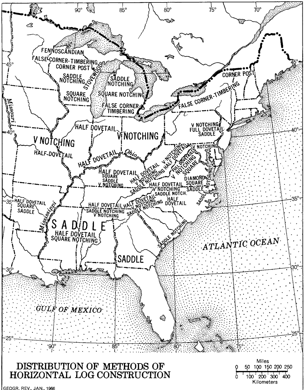
FIG. 28—Distribution and dominance of methods of horizontal log construction. Based on approximately one thousand individual examples. Differences in weight of terms are indicative of relative importance.
