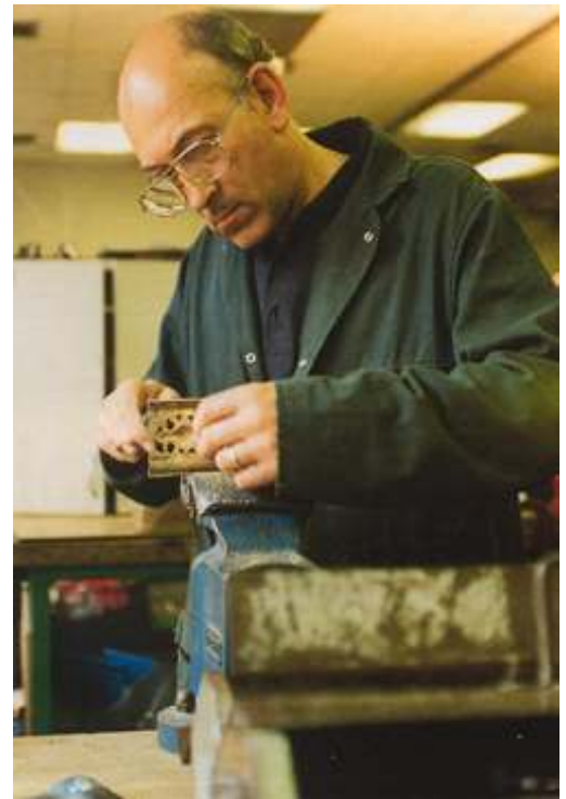
A craftsman at Denmans Montrose Ltd cleaning the 'flashing' or mould lines from a cast replacement for the 'gallery' of a light fitting. Originally stamped from very thin metal, the cost of making a new stamp for individual repairs is prohibitive, and individual replacements have to be cast from moulds made from the original component.
