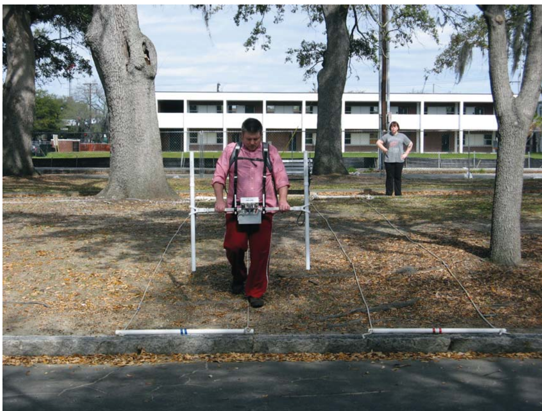
Figure 2. Jon Marcoux walking transects with the magnetic gradiometer at Wragg Mall.
