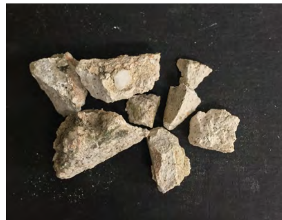
Figure 18: Detail of bulk sample with visible shell aggregate.
