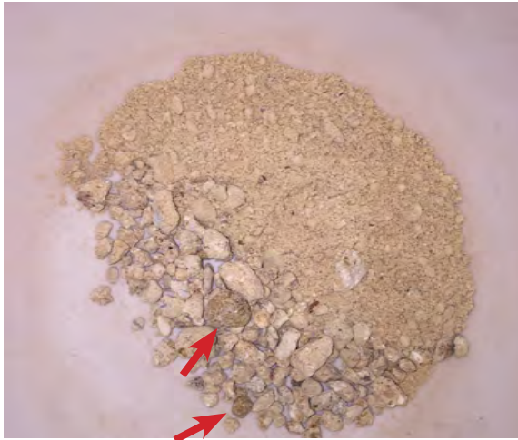
Figure 7: Powdered sample prior to addition of acid. Note round brown clay lumps within mortar (arrow).
