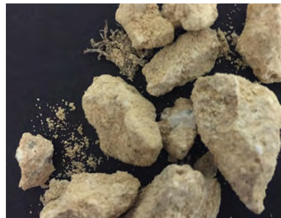
Figure 4: Close-up of bulk sample showing numerous shell fragments.
