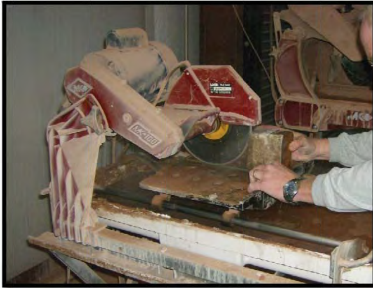
Figure 3.5: Cutting brick samples with the tile cutter. (Lanphear)
