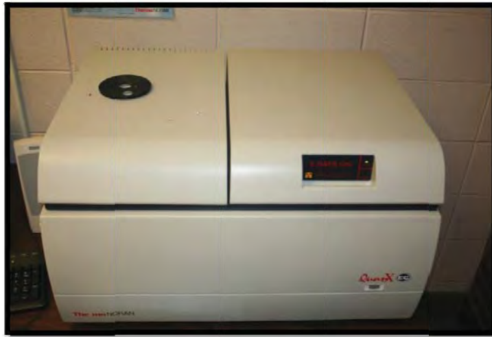
Figure 3.9: X-ray Fluorescence Instrument; QuanX EC XRF, by Thermo Noran. (Lanphear)
