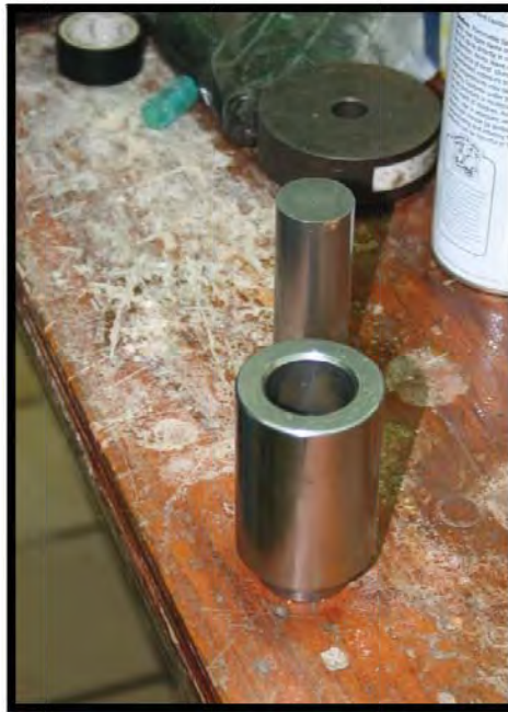
Figure 3.17: The mold that created the disks for the thermal gradient firing. (Lanphear)
