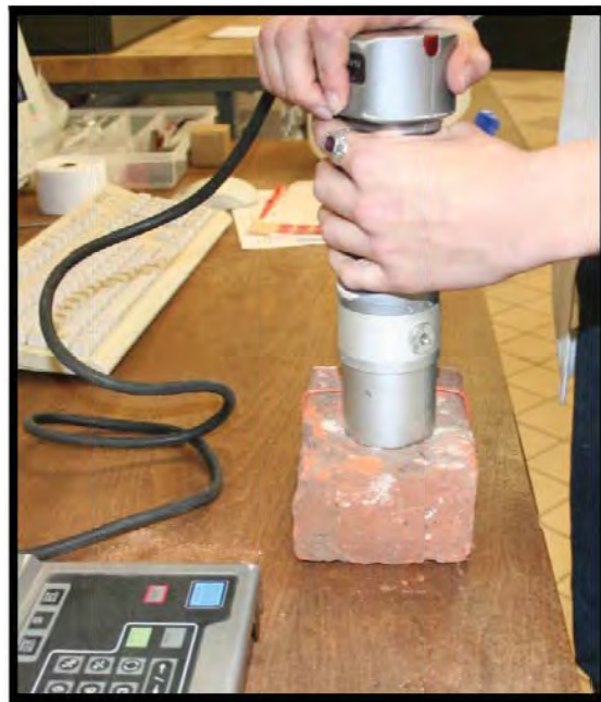
Figure 3.24: Colorimeter Instrument. Manufactured by Minolta. (Michael Mason)
