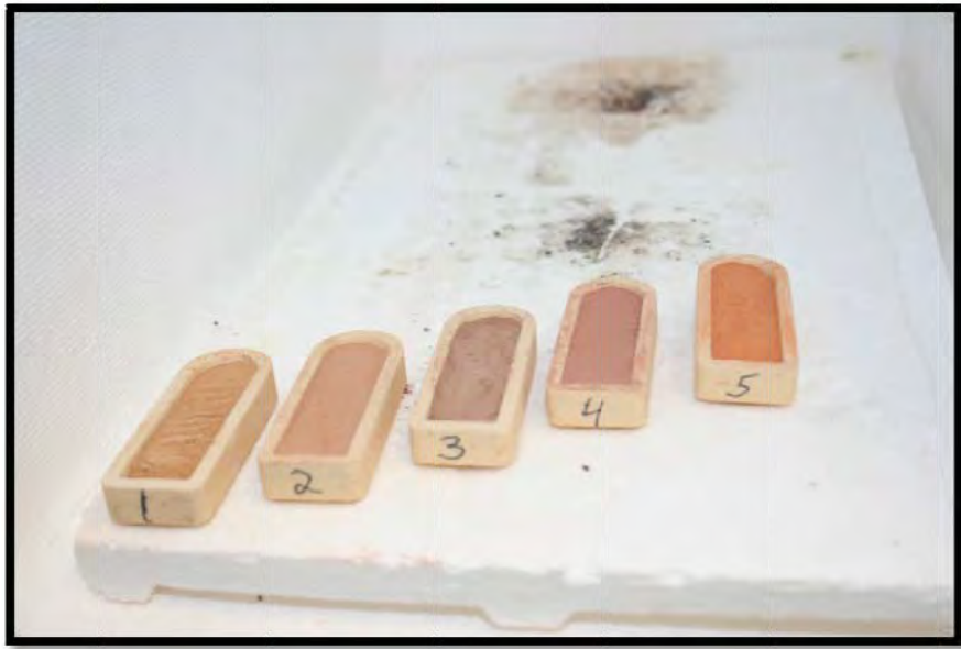
Figure 3.7: Five of the brick samples in the oven for the Loss of Ignition test. (1) Lord Ashley, (2) Dorchester 1091, (3) Dorchester 1067, (4) Dorchester 1428, & (5) Drayton Hall 1118. (Lanphear)
