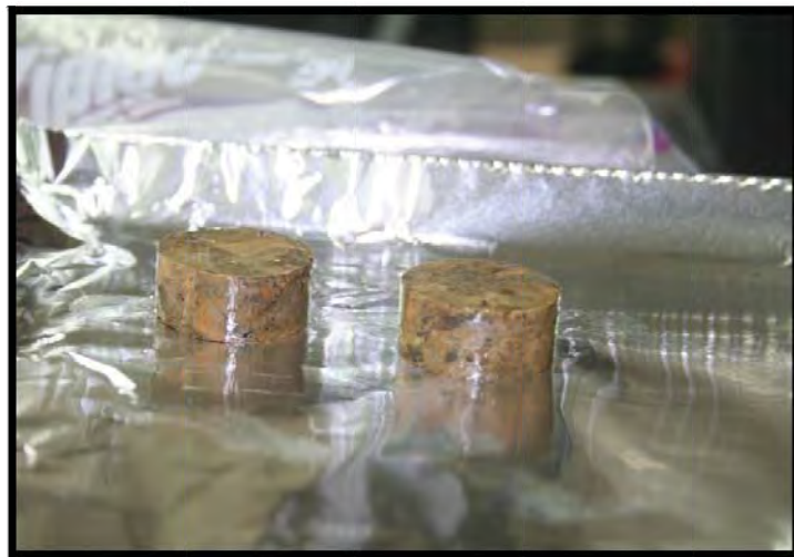
Figure 3.18: Example of two disks from Church Creek clay sample. Ten disks are made for each clay sample. The color is examined before and after the firing. (Lanphear)
