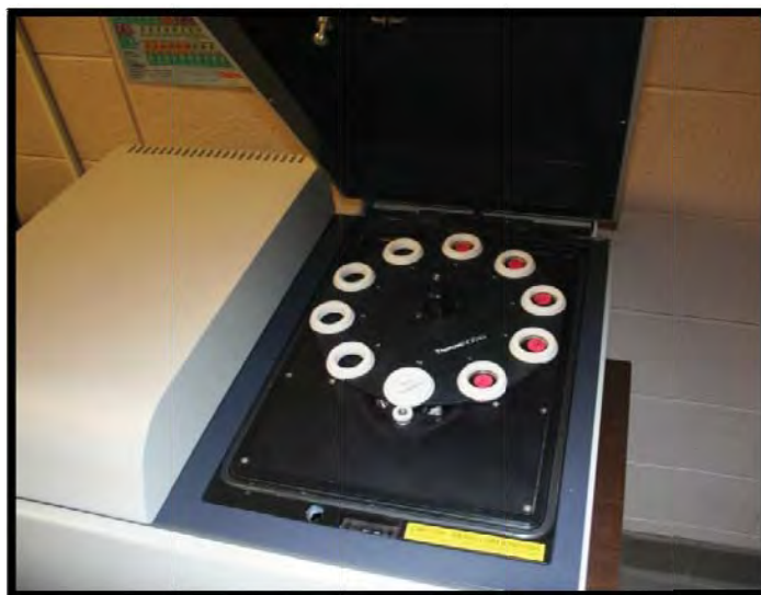
Figure 3.11: Five samples in the XRF instrument. This XRF can read ten samples in a short time. The elements are then reported through the computer program. (Lanphear)
