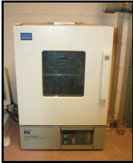
Figure 3.23: Dryer used for moisture content testing. Scientific Product: Gold Series. (Lanphear)
