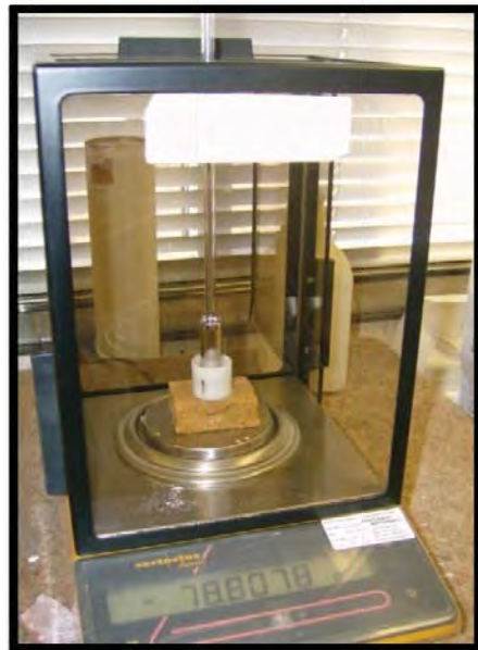
Figure 3.14: Weighing the sample after the mercury intrusion test. The entire tube is filled with mercury and the sample. (Lanphear)
