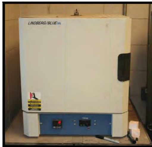
Figure 3.8: Small electric kiln for heating in Loss of Ignition test. Lindberg/ Blue oven. (Lanphear)
