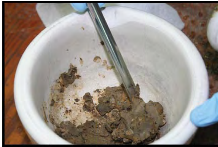
Figure 3.16: The clay sample was mixed with a little water to form a paste. A mortar and pestle are used. (Lanphear)
