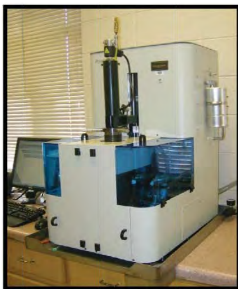
Figure 3.12: Mercury Intrusion Porosimeter. Produced by Quantachrome PoreMaster. (Lanphear)
