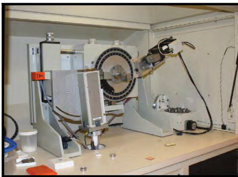
Figure 3.1: X-ray Diffraction Instrument; XGEN-4000 made by Scintag. (Lanphear)
