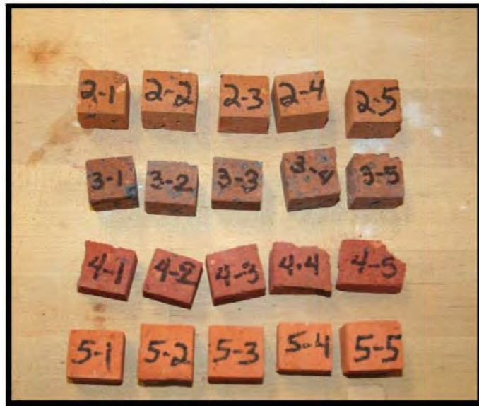
Figure 3.21: The three samples were cut into five one-inch cubes. (Lanphear)
