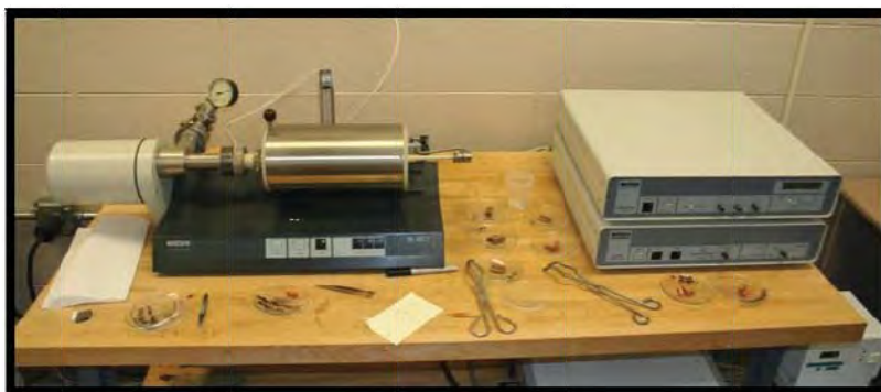
Figure 3.4: Thermal Expansion Instrument/ Dilatometer. Netzsch DIL 402 C Dilatometer. (Lanphear)
