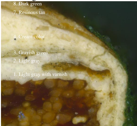
Sample S201-8. South wall, east window, rail below transom window Visible Light 200X
