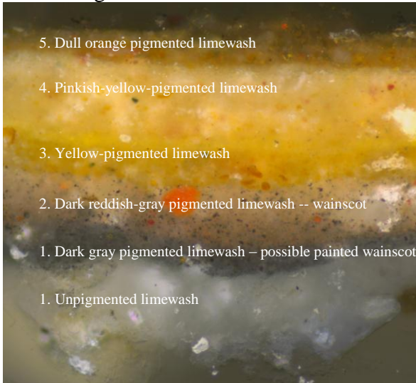
Sample S103-1. East wall, crude board wall about 5' up.
