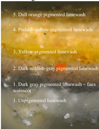
Sample S103-1. Crude board wall Visible Light 200X
