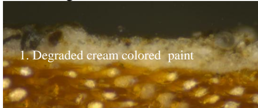
Sample K103-II-3. Staircase, newel post Visible Light 200X
