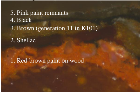
Sample K203-II-4. West wall pegrail, lower edge for comparison of paint chronology. Visible Light 200X
