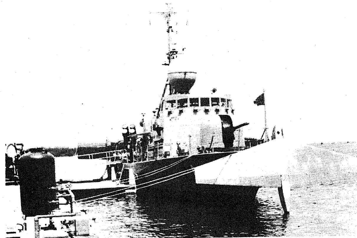
A hydrofoil with foils raised, showing the wing-like device at the front and rear.
