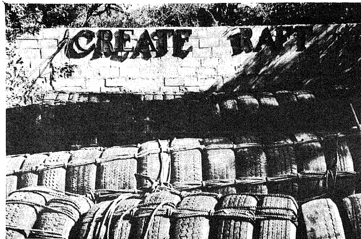
Tires filled with plastic bottles and styrofoam, then lashed together, are the building blocks for a raft which is scheduled to float from Key West to Hamburg, Germany. Photo by Christopher Weiland.
