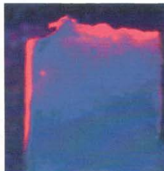
Image 12. Nanoparticle/Consolidant– Matrix Compatibility Test Evident T2 EviDot™ Maple Red-Orange & Paraloid B72 applied to a marble sample under ultraviolet light (350nm).
