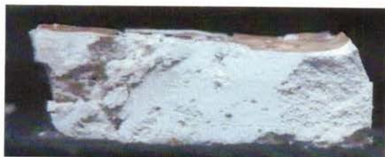
Image 4. Crossection Mural mockup treated with Isinglass tagged with Sun Innovations™ YVE1005 under halogen light. 100x magnification
