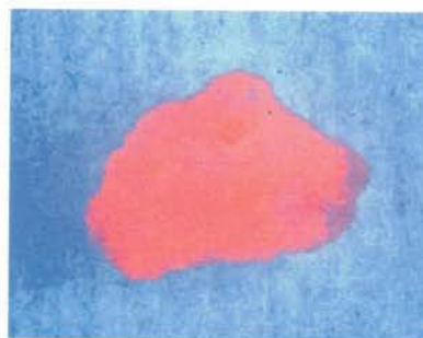
Image 16. Nanoparticle/Consolidant– Matrix Compatibility Test Evident T2 EviDot™ Maple Red- Orange & Paraloid B72 applied to a sugar cube under ultraviolet light. Unconsolidated material has been removed. Entire sample fluoresces.
