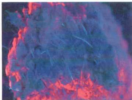
Image 11. Nanoparticle/Consolidant– Matrix Compatibility Test Evident T2 EviDot™ Maple Red-Orange & Paraloid B72 applied to a plaster sample under ultraviolet light (350nm).
