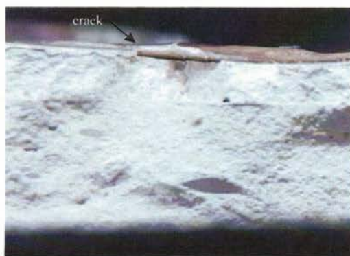
Image 6. Mural mockup treated with Paraloid B72 tagged with Evident T2 Evi Dot™ Maple Red- Orange under halogen light. 100x magnification
