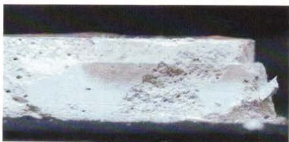
Image 2. Crossection Mural mockup treated with Paraloid B72 tagged with Evident T2 Evi Dot™ Maple Red-Orange under halo- gen light. 100x magnification
