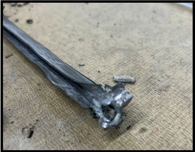
FIGURE 10: Views of hollow heart lead came
