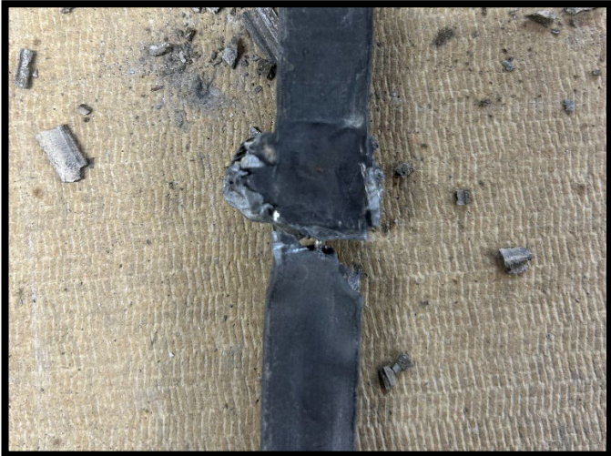
FIGURE 10: Views of hollow heart lead came
