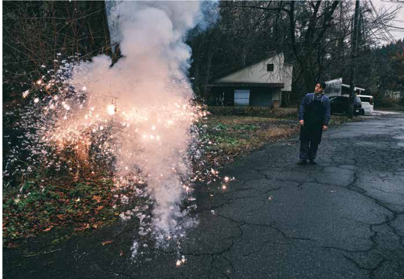
Above, a technician tests the “tail” of a firework—the streak you see as the firework shell ascends before it bursts. They are trying to create a four-second tail—four seconds between launch and explosion. Facing page: A display in Winter Fantasy in Nagaoka.
