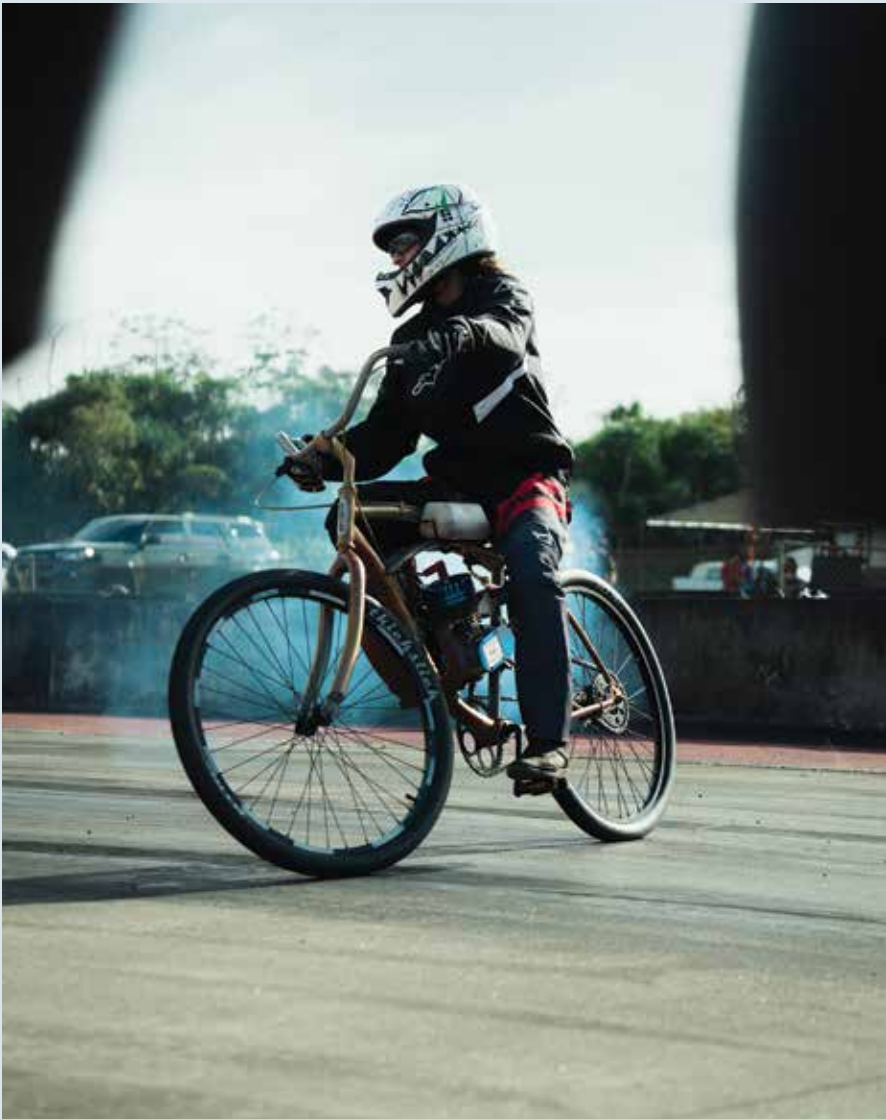
Tanya Davis revs up on Whirlwind , a gas-powered bike built by her husband, Neill C. Davis Jr. (seen on pages 20-21), at Hilo Drag Strip. The 1970s Schwinn beach cruiser, modded with a seventy-five-cc engine, clocks over fifty-five mph.
