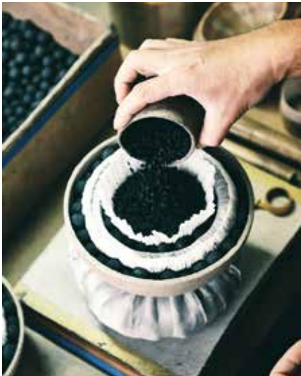
OPENING SPREAD / “Stars” are at the heart of fireworks. They are created by applying layers of a black powder slurry—a combination of explosives and metals for color—in a rotating drum. Here, the stars are sifted at Abe Fireworks in Nagaoka, Japan, to ensure they are of uniform size.
