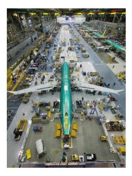
A Boeing 737 MAX sits in the first position on the Renton plant's new production line, where mechanics are refining the production process.
