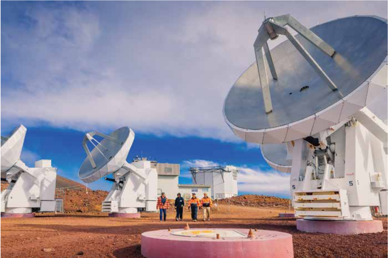
Technicians walk among three of SMA's eight robotic receivers, which can be positioned in specific patterns to optimize observing cold, gaseous bodies and black holes; SMA was one of many radio telescopes that provided data for the first images of a black hole in 2018.
