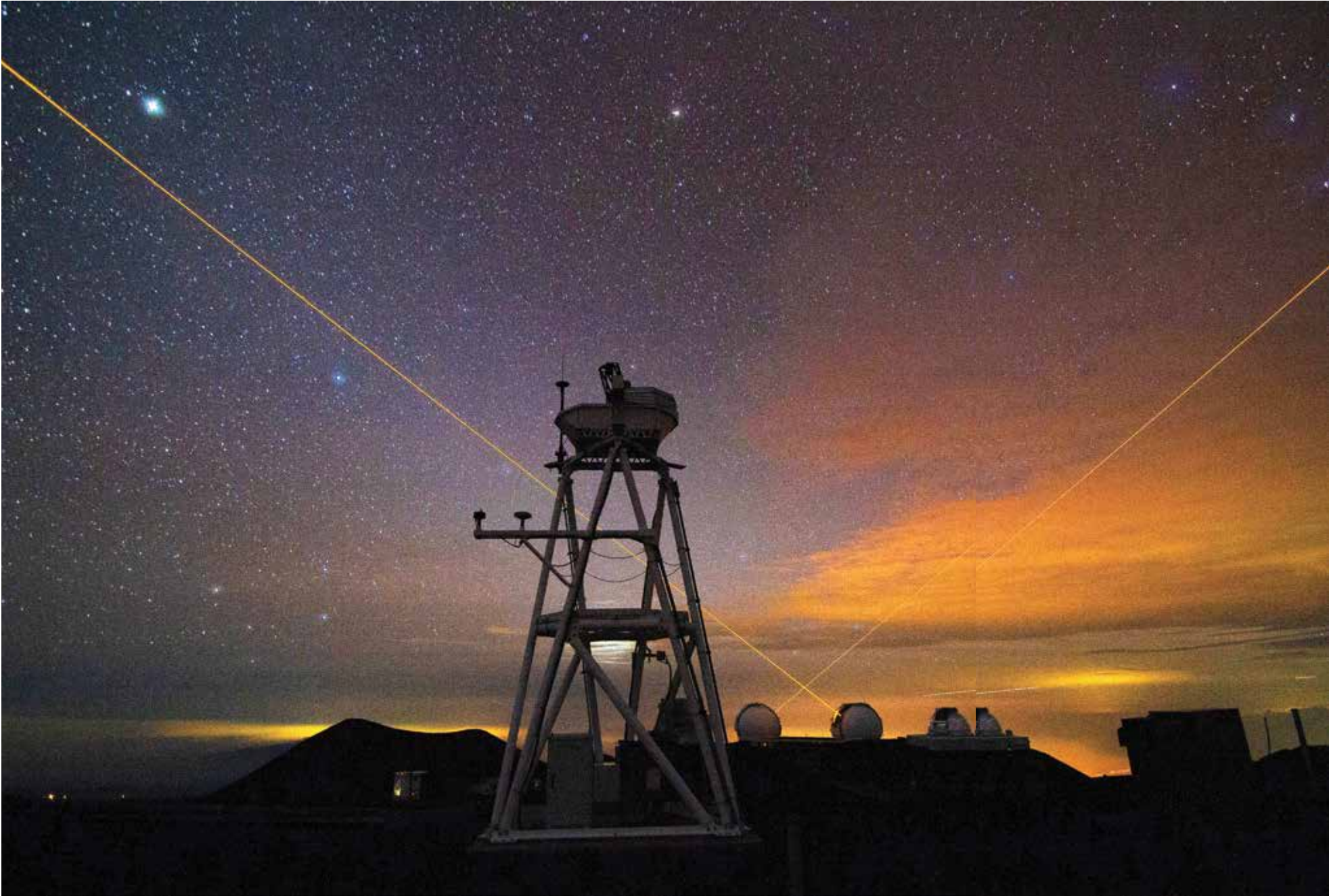
The WM Keck Observatory fires twin lasers to create “artificial stars” in space to help pinpoint the telescope. For optical telescopes like those at Keck, MKWC provides critical information about cloud cover and high-altitude winds that distort observations even on clear nights.
