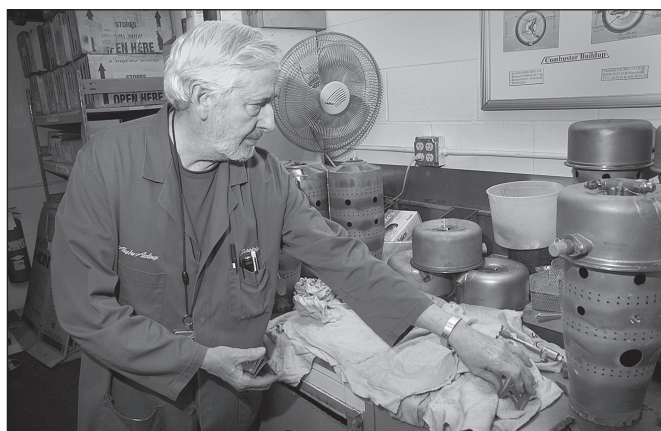
Aircraft Technician Earle Partain cleans the "burner cans" from an auxiliary power unit.
