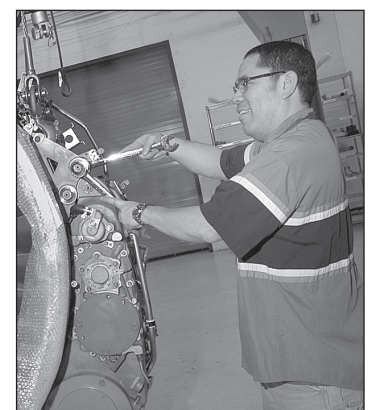
Aircraft Technician Gordon Mimura uses a pair of wrenches to simultaneously tighten and loosen bolts.
