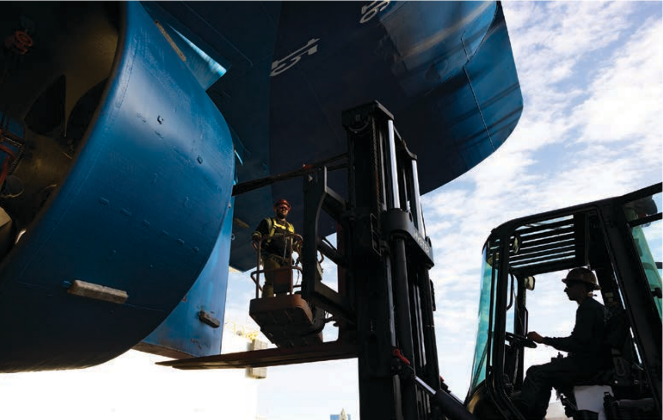
Shipyards workers finish reinstalling MV Carolyn Chouest ’s massive rudders. Repairs are usually carried out at Pier 24 in Honolulu Harbor, but the dry-dock system is mobile and can be towed to where it’s needed.
