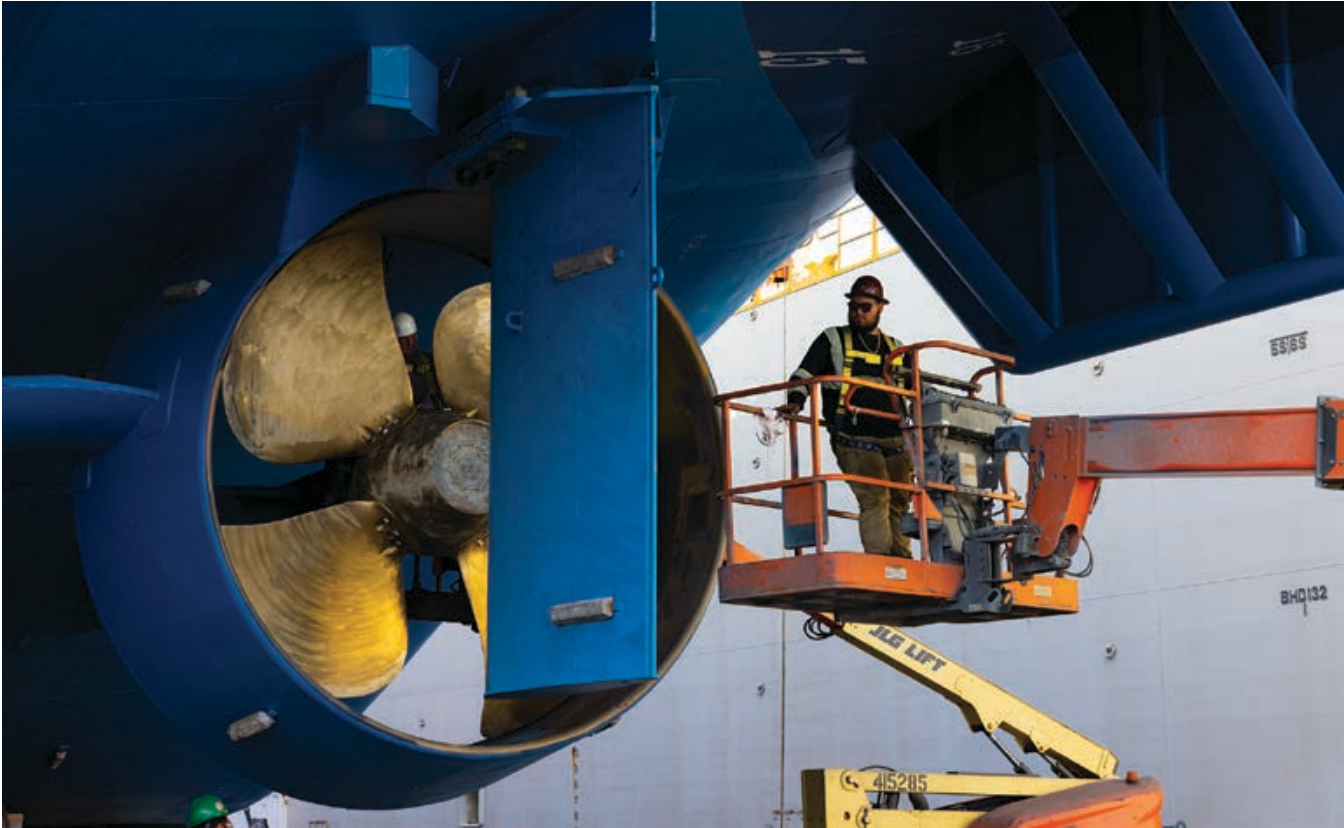
Mechanic Zach Meyers stands on a telescopic boom during a quality-control check following the reinstallation of MV Carolyn Chouest’s shafts, propellers and rudders. Once repairs are complete, the dry dock’s platform will be lowered and the berth flooded, allowing the ship to float off the support blocks and return to service.
