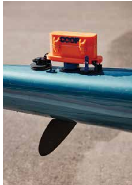
ABOVE / Engineered by Mark Baldwin at the University of California, Irvine, CoOP's motor attaches to a canoe's rudder, which is typically controlled by the paddler using foot pedals. A sighted steersman navigates with a remote control dial.
