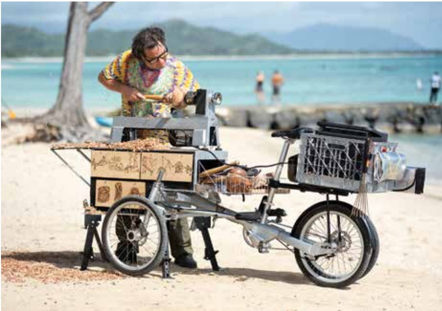
Wood artist Aaron Hammer turns a bowl at Kailua Beach. Seeking to escape the confines of his studio, Hammer built the battery-powered, trike-mounted mobile lathe seen above.
