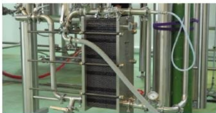
The heat exchanger gives a master brewer more precise control when cooling down wort.
