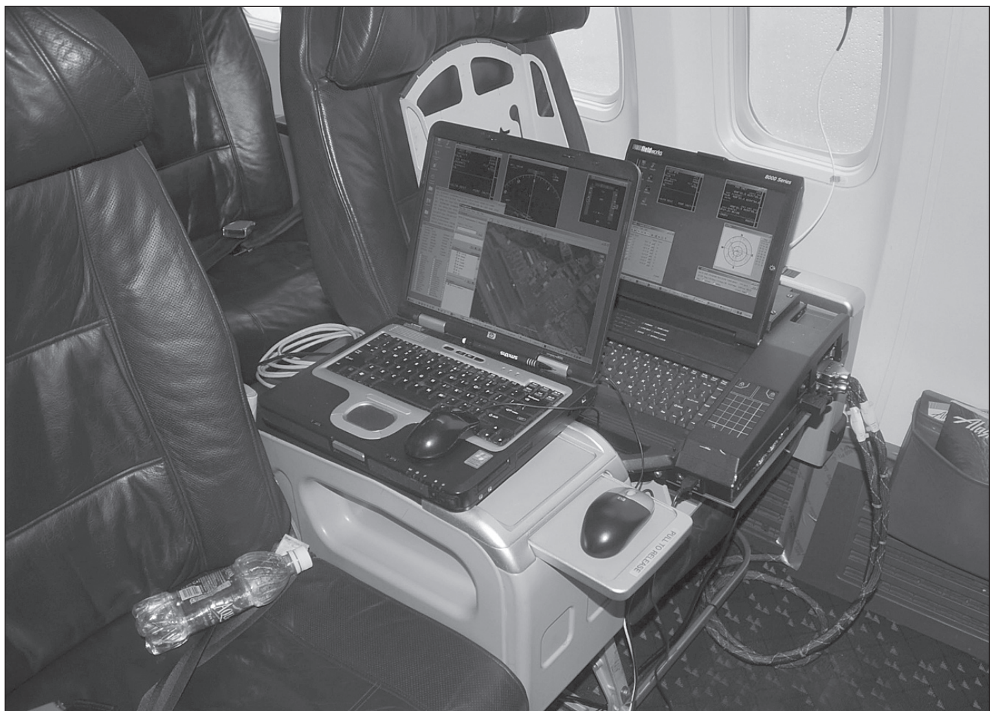
Empty passenger seats hold computers and other equipment during RNP test flights.
