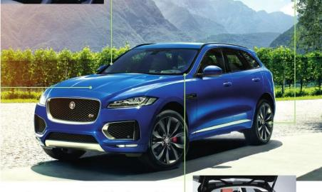
Two engines are available: a strong, economical turbo-diesel making 180 hp, and a 340-hp or 380-hp supercharged V-6. Both come with a smooth. responsive eight-speed automatic transmission. The turbo-diesel's strong 318 lb-ft torque rating (versus 332 lb-ft for the V-6) makes it nearly as quick as the V-6, and it returns an EPA combined 29 mpg (versus 20 for the V-6).
