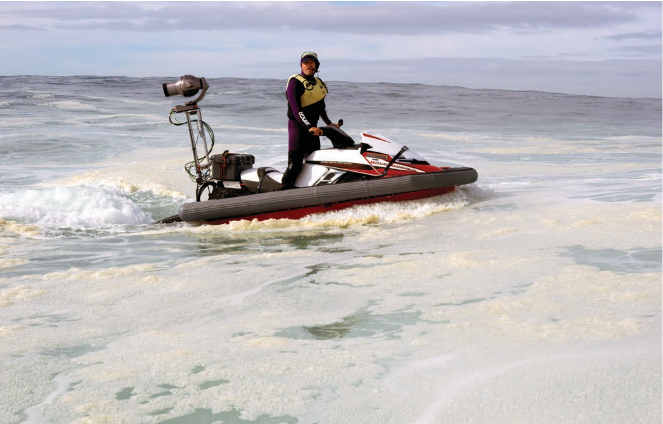
To capture the raw power of Nazaré (seen on the previous spread) for 100 Foot Wave , Prickett designed a jet ski-mounted, gyro-stabilized gimbal camera (seen above, with driver Alemao de Maresias), which he controls remotely while directing the driver. “This is a ground-breaking invention that has never been tried before in massive surf,” says Prickett. Shooting Nazaré from the water toes a fine line between perfection and a pummeling, leaving only seconds for the driver to outrun an ocean-going avalanche with a $500,000 camera—and his life.
