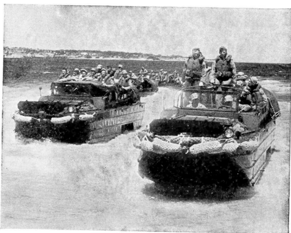
GM builds the "Duck," an amphibious vehicle which permits new tactics in landing operations.
