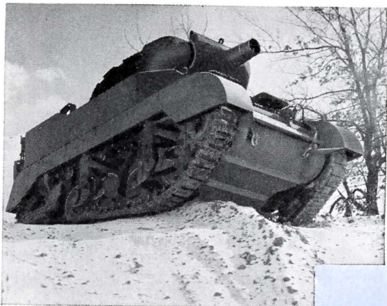
The new GM-built M-8 howitzer motor carriage uses the M-5 tank chassis and GM motive power and Hydramatic transmission.
