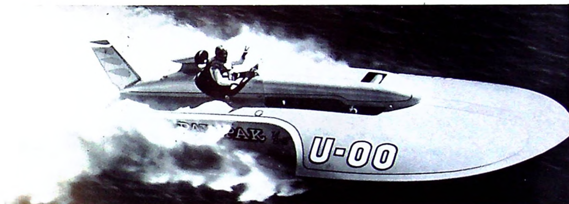
U-00 Pay 'n' Pak's Lil Buzzard - Owned by Dave Heerensperger Built by Staudacher. Length 30'; Width 12'; Weight 6,500 lbs. Rolls Engine.
