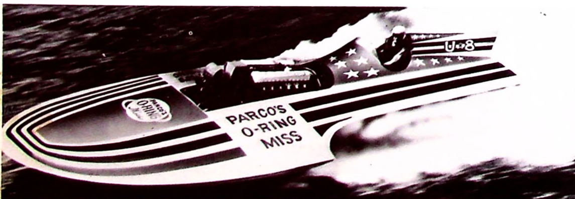
U-8 Parco O-Ring Miss - Owned by Laird Pierce Built by Karelson. Length 30'; Width 13' 2"; Weight 5,500 lbs. Rolls Engine.
