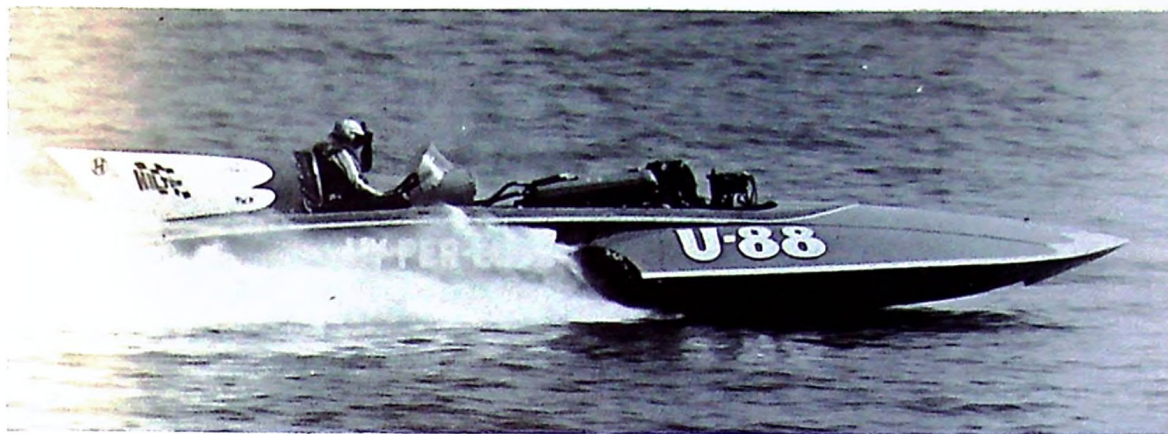
U-88 Fascination - Owned by Bob Gilliam, Seattle, Wash. Built by Gilliam. Length 32'; Width 12'; Weight 7,000 lbs. Rolls Engine.
