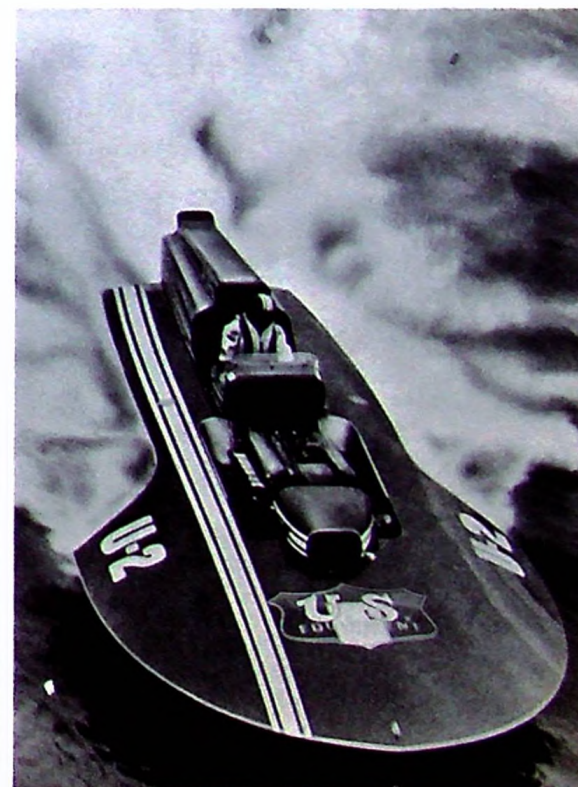
U-2 Miss U.S. - Owned by U.S. Equipment Company Built by Staudacher. Length 30'; Width 12'; Weight 6,500 lbs. Rolls Engine.
