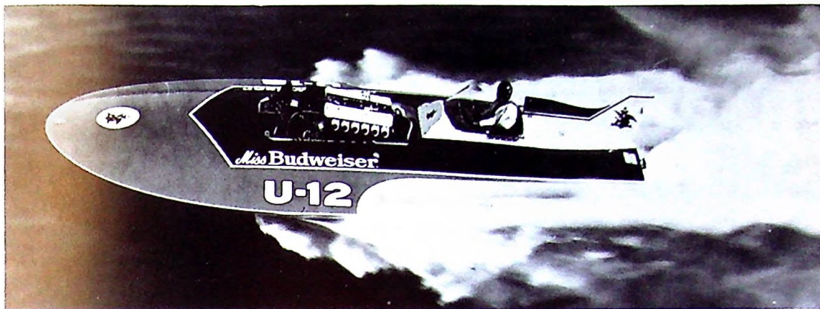
U-12 Miss Budweiser - Owned by Hydros, Inc. Built by Karelson. Length 30'; Width 13' 2"; Weight 7,000 lbs. Rolls Engine.
