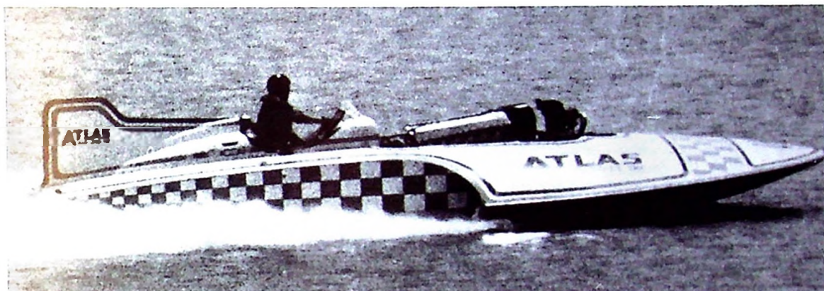
U-19 Atlas Van Lines owned by Bob Fendler Built by Staudacher. Rolls Engine. 29'6"x12'. 5,700 lbs.
