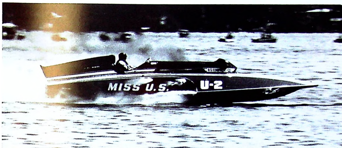
U-2 Miss U.S. owned by U. S. Equipment Company - Driven by Bill Muncey Built by Staudacher. Rolls Engine. 30'x13'2". 6,900 lbs.
