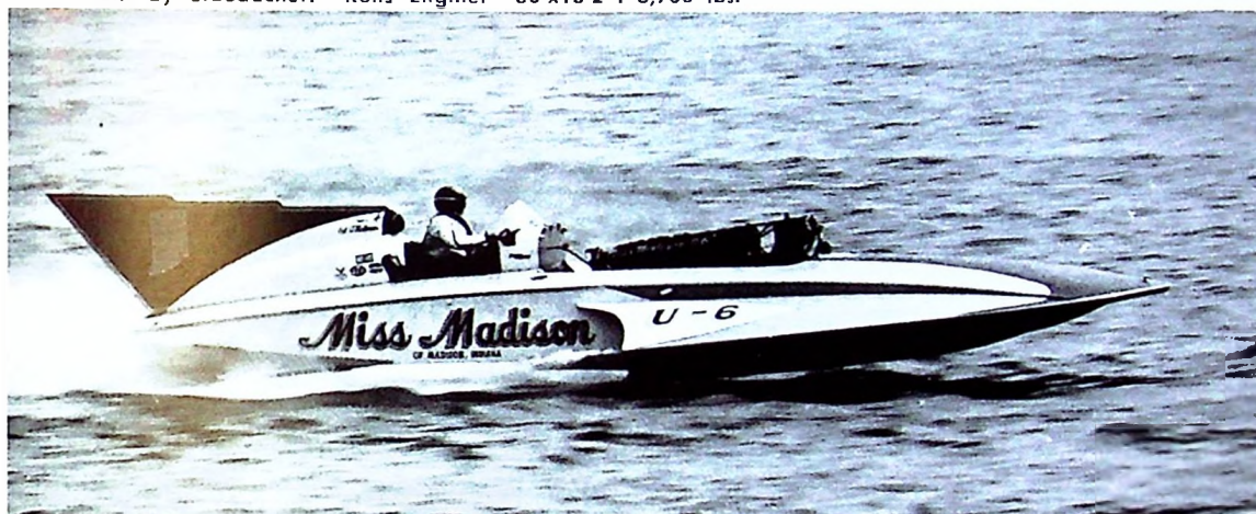
U-6 Miss Madison - owned by City of Madison, In. - Driven by Jim McCormick Built by Staudacher. Allison Engine. 30'x12'. 6,600 lbs.
