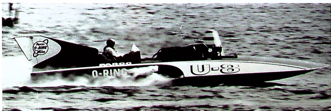
U-8 Parco-O-Ring Miss owned by Golden State Racing - Driven by Norm Evans Built by Patterson. Rolls Engine. 30'x12'. 6,750 lbs.
