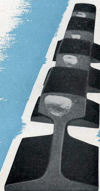
Here are examples of internal rail defects invisible to the eye but found by the rail G-men
