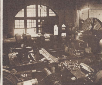
This machine is used for turning large crank pins in Hoboken Yard, Shipbuilding Division, Bethlehem Steel Company.
