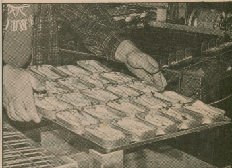
Trays containing 25 cans of packed fish are then loaded onto portable carts and taken to the steam box for a first cooking. Sauces are then added, the cans are sealed, and the fish are cooked again. 8
