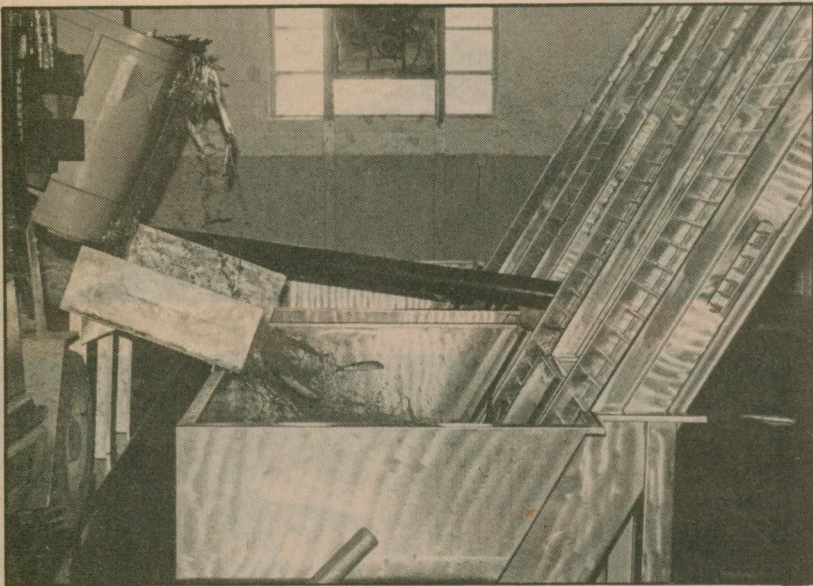
At the Prospect Harbor plant of the Stinson Canning Company, fresh or frozen fish arrive in tote boxes that are then emptied into the loading bin of the sorter which is part of the new automated equipment recently installed there. 1.
