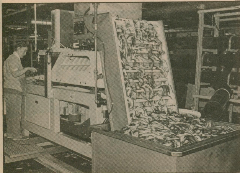
Fish are delivered to the six new cutting machines through an arrangement of pipes, and a conveyor then lifts the fish to a vibrating table where they are lined up for the cutters. 3.
