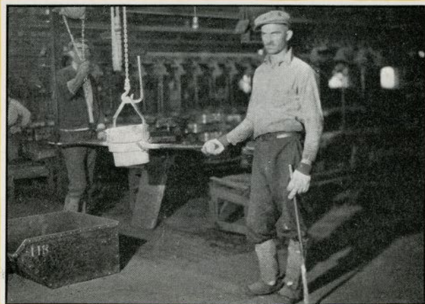
An efficient monorail conveyor system expedites the handling of molten metal, conserves the workman's energies for more important tasks, and increases production.
