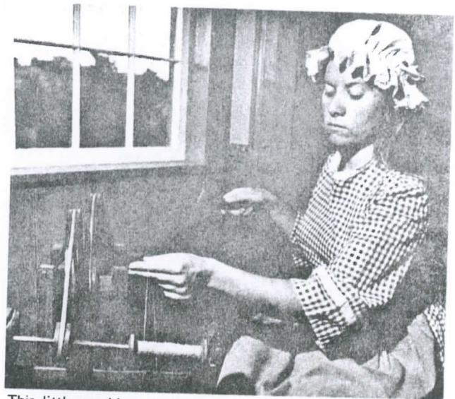
This little machine winds spools used in making a warp. It consists of three pulleys connected from two circular leather belts. Turning the handle one revolution makes the spool turn 16 times and winds on approximately 45 inches of thread.
