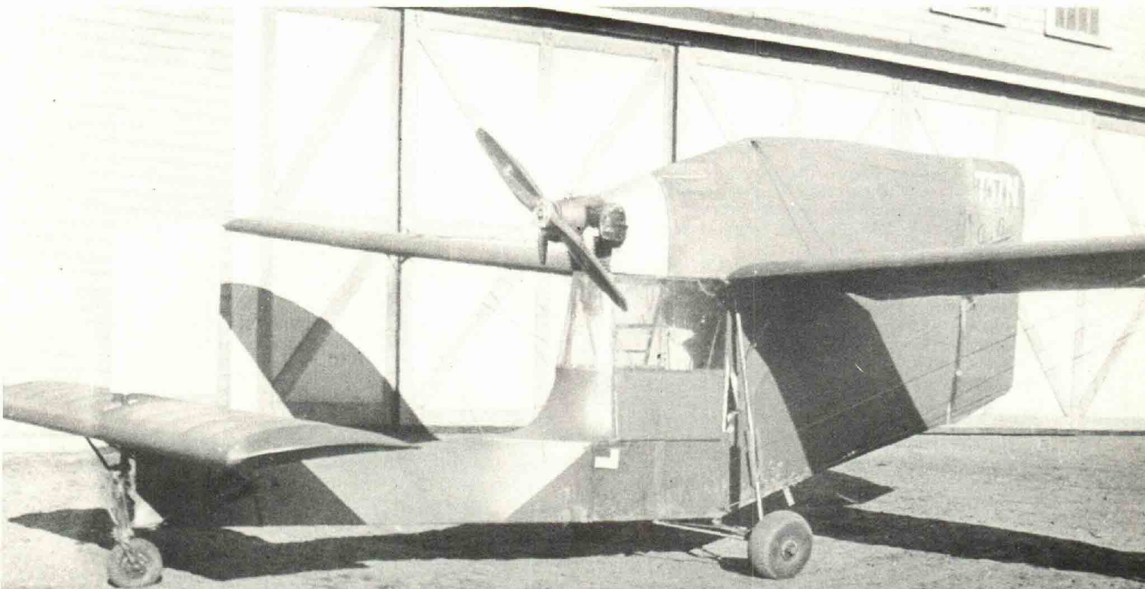
The Gee Bee Ascender, a test bed for a roadable aircraft concept. The strange little canard flew well, but suffered from poor aileron response — likely from the fact that the wing was from an Aeronca C-2, which shared that characteristic. The 2-cylinder Aeronca engine was also from a C-2. The aircraft was heavily damaged in a landing accident and was never rebuilt.
