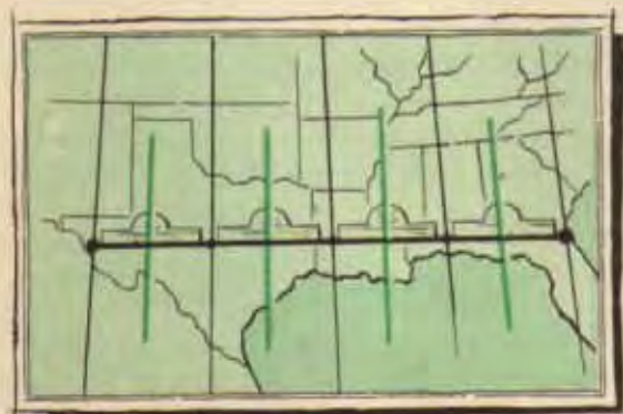
DIVIDE FLIGHTS MORE THAN 500 MILES INTO LEGS AND MEASURE EACH AT ITS MID-MERIDIAN
