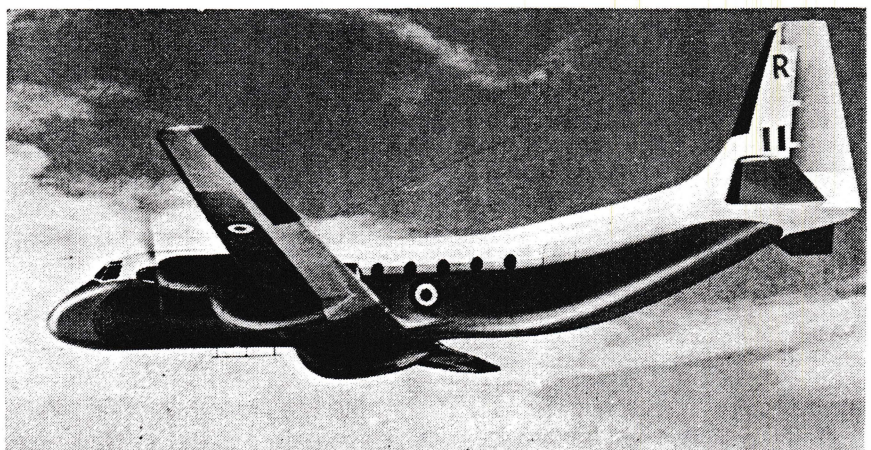
HAWKER SIDDELEY AVRO 748, which has been ordered for the Royal Air Force, has an undercarriage system that can be adjusted vertically and horizontally to align the fuselage floor of the rear-loading aircraft with bed of loading vehicle. The military version is the Dart 12-powered Avro 748 MF, which will carry 48 fully-equipped troops or 14,000 lbs.
