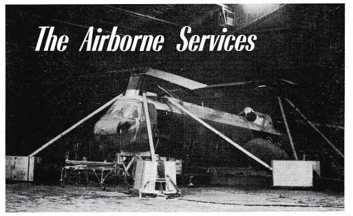
**NEW VERTOL CH-113 SEARCH & RESCUE** helicopter for the RCAF recently completed cold weather tests at USAF's Eglin AFB climatic hangar in Florida. The RCAF has ordered six CH-113's, which are basically the same as Vertol 107. CH-113 is specially equipped for long range northern operations.
