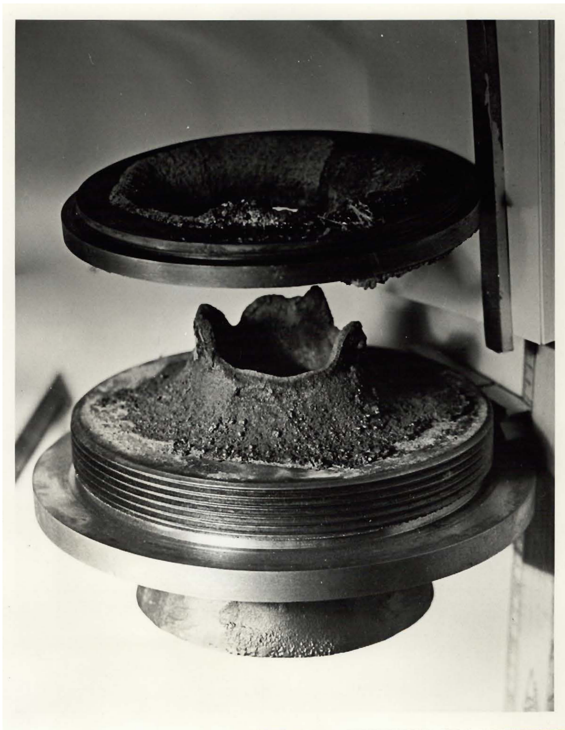
MEEHANITE NOZZLE AFTER FIRING N5 - ALUMINIZED MOTOR
