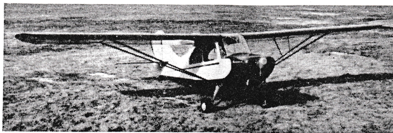
AERONCA CHAMPION: The new Aeronca Champion Model 7EC-90 hp electrical model airplane incorporates flush type locking door handles and locking left sliding windows as standard equipment. It has a full width rear seat and a high output cabin heater. The new Champions are painted Packard Straw and Sedan Red. As standard equipment the aircraft also have Aeronca's no-bounce landing gear and stall warning indicators, as well as generator, starter, navigation and landing light wiring.
