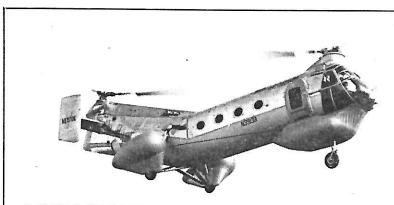
AMPHIBIAN HELICOPTER: Vertol Aircraft Corp., has combined fuselage sealing with newly designed flotation gear to make an amphibian helicopter. Above: Watertight fuselage and three rubberized fabric floats permit the Vertol 44 to land on water in an emergency. Below, left: Landing at 30 knots, 'copter feels like a flying boat. Below, right: Pilot takes off from water just as he would from heliport.
