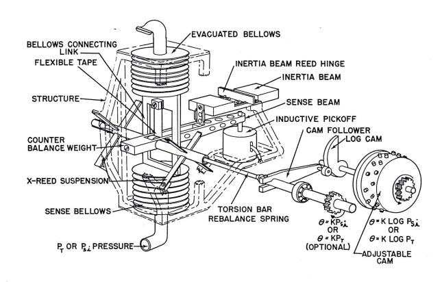
Figure 2. Transducer Schematic
