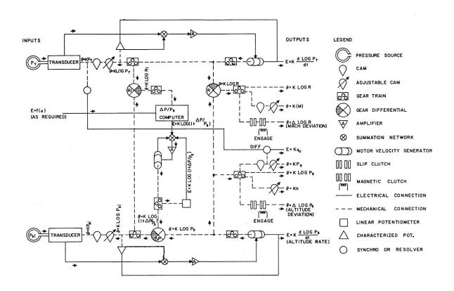
Figure 3. Detailed Schematic Diagram of Mechanical Computer Section (Pressure Data Section)
