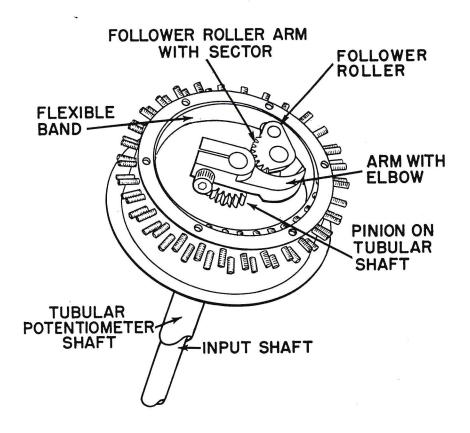
Figure 4. Adjustable Cam
