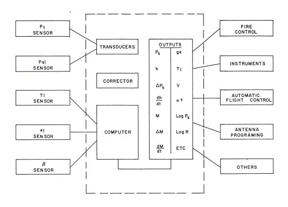
Figure 1. Block Diagram - Basic Air Data System
