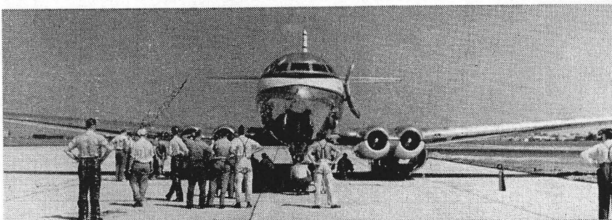
ABOVE — Close-together location of engines and short undercarriage, made possible by absence of props. are evident here.
