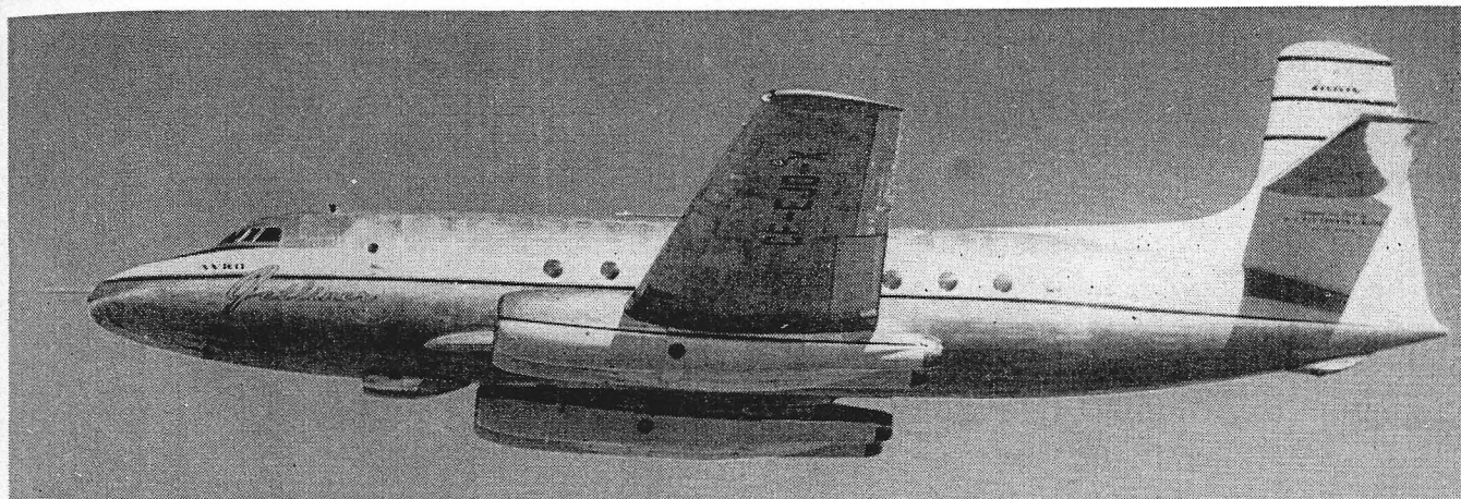
ABOVE — Trim lines, tapered wings, underwing nacelles and high-set tailplane are apparent in this profile view of the Jetliner in flight.
