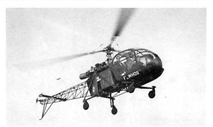
ALOUETTE JET HELICOPTER: The jet helicopter Alouette which Republic Aviation Corporation will market in the U.S. The five-place, medium-range (345 miles) Alouette is propelled by the 360 hp Artouste IIB-I turbine engine produced by Turbomeca of France. The Alouette is 32 feet long, 9 feet high, and its main, three-blade rotor has a diameter of 23½ feet.
