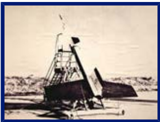
Early aerodynamic data on the Arrow design was gathered from small wind tunnel models and larger free flight models mounted on Nike rockets. 16
