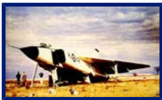
Not all test flights proceeded without incident. Both Arrow 201 and 202 suffered minor damage when they crashed on landing due to collapse of the landing gear. 27
