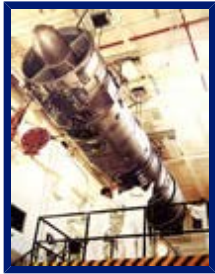
Another subsidiary of A.V. Roe Canada Limited, Orenda Engines Limited designed the Iroquois jet engine as the intended powerplant for all production Arrows. The Iroquois remains one of the most advanced jet engines ever developed. 58
