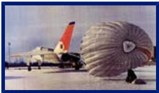
Arrow 203 with drag chute deployed. The drag chute brought the aircraft to a quick stop upon landing. 28
