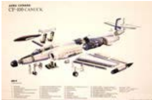
Exploded view showing the major components of the Avro CF-100 Canuck Mark 4. 10
