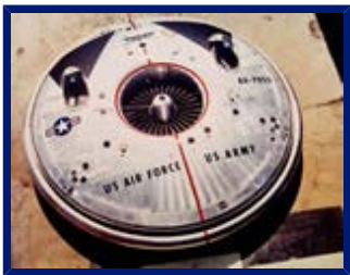
With the termination of the Arrow programme, Avro was left with few contracts. One was for the Avrocar, a vertical take-off and landing circular-wing air-cushion vehicle. A United States Air force funded project, it too was cancelled in 1961 after ten unsuccessful years of research and development. 76
