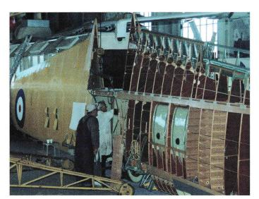
struction of the wing and spars required a jig table 60 feet long which we made and leveled. As is typical of modern spars, the caps (or booms) were laminated. A band-saw at SAIT was a big help in cutting 1400 linear feet of laminating material from the sitka timbers we had previously obtained.
