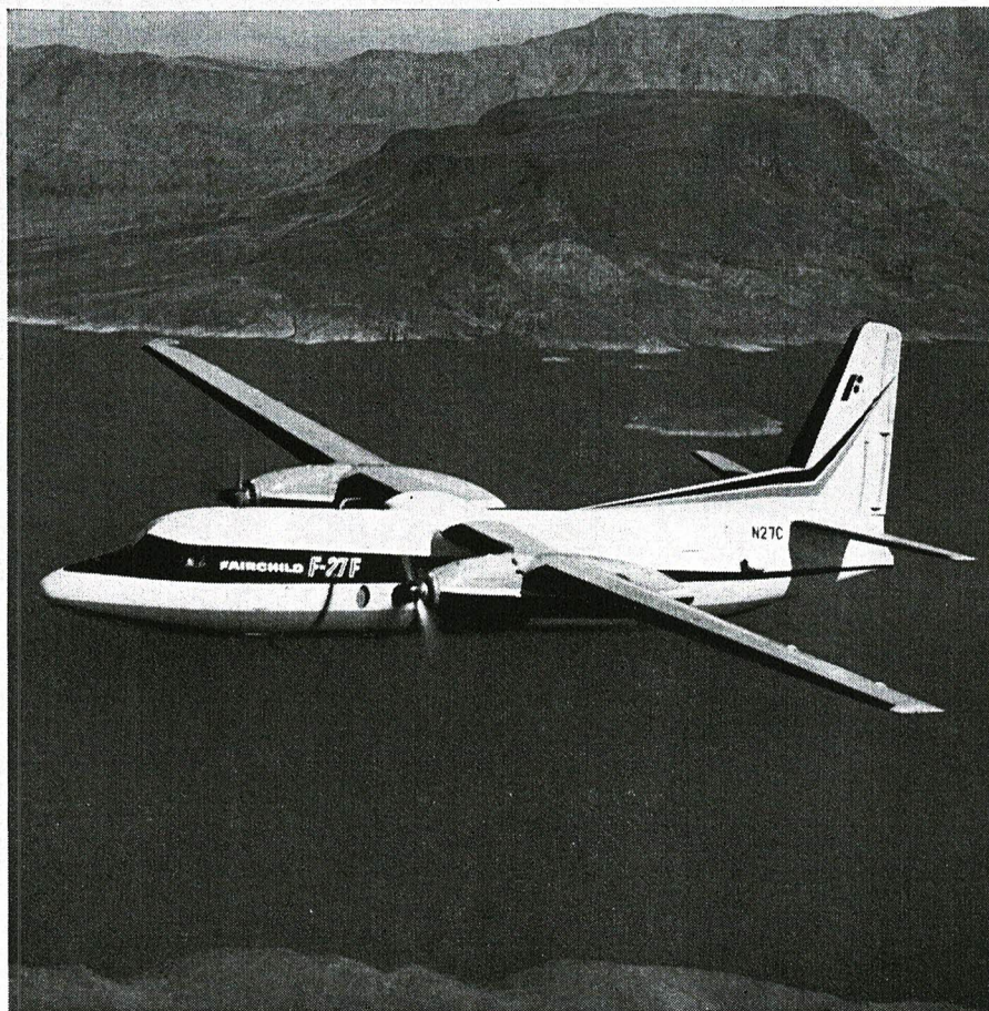
Fairchild Stratos Corporation's F-27, now serving twelve airlines and twenty-five corporations . . . as transport, executive plane and mixed cargo transport. Complete pneumatic system is actuated by air stored at 3300 psi, and provided through two engine gear box driven 2 cfm air compressors.
