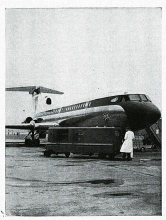
The HOUCHIN "RECTI-HY-CY" aircraft Starting and Servicing Ground Power Unit is capable of the following outputs:
