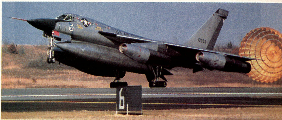
During a B-58 landing, a high angle of attack was maintained as long as possible to act as aerodynamic braking. The drag chute was deployed just after touchdown (photo by Ken Smith, courtesy of Warren Thompson).
