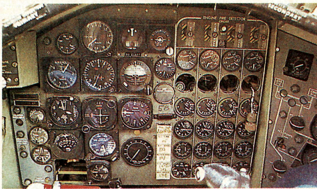
The B-58A's innovative, pilot instrument-panel layout was far ahead of its time: every knob, toggle and switch came easily to hand (Mick Roth, courtesy of author).
