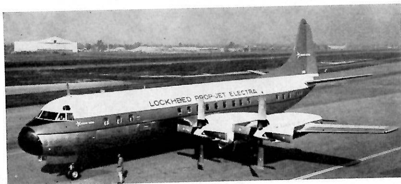
MAIDEN FLIGHT FOR ELECTRA: The Lockheed Electra took to the air for the first time December 6, remaining airborne for 1 hour 26 minutes. The aircraft flew 56 days ahead of the original target date of January 31. Designed for operation on short-to-medium range routes, the turboprop Electra cruises better than 400 mph carrying from 66 to 91 passengers. It has 99-foot span, is 104 feet long. It is powered by four 3750-hp Allison Model 501 turboprop engines.
