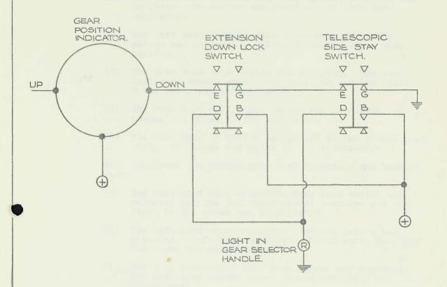
SCHEMATIC OF MAIN LANDING GEAR ELECTRICAL SYSTEM-COCKPIT INDICATOR.
