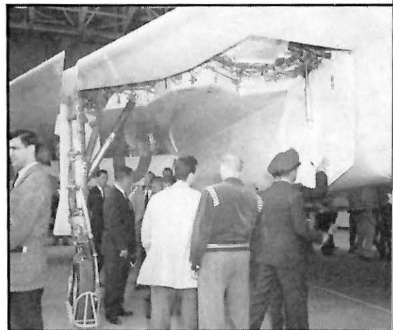
Main undercarriage twists and shortens when retracting. Main gear is by Dowty; nose gear by Jarry. Note extended and notched leading edge. Depth of wheel well is indication of wing's extreme thinness.
