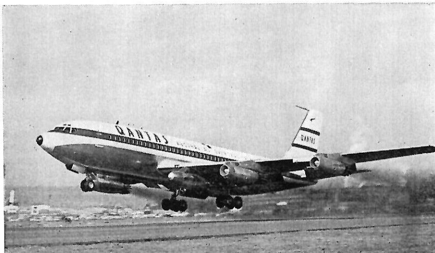
707 WITH FIVE. Carrying spare power plant in left wing Pod-Pak, a Qantas 707 lifts off for a test flight. Handy Pod-Pak is an optional feature of the Boeing jet.
