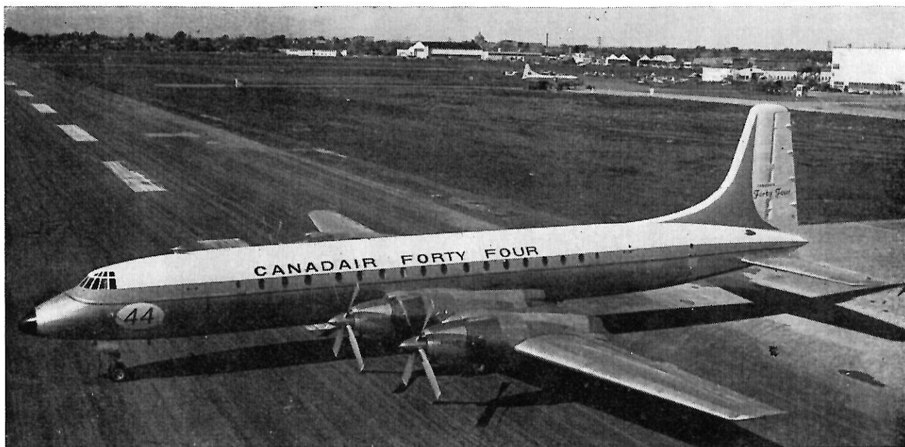
NUMBER ONE. Canadair's Forty Four, first of 12 of R-R Tyne powered transports being built for RCAF is completed and preparing for first flight sometime this month. Orders have been received for 17 hinged-tail commercial versions of aircraft.
